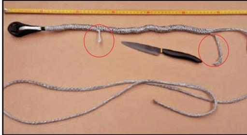
11/ Smooth the splice in order to make the Dyneema<sup>®</sup> cover and the taper go inside the textile cable. You should obtain the same system as below.
