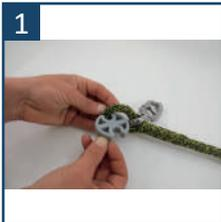
1/ Place the halyard stopper with its narrowest side onto a spliced eye and insert the eye in the lower groove.
