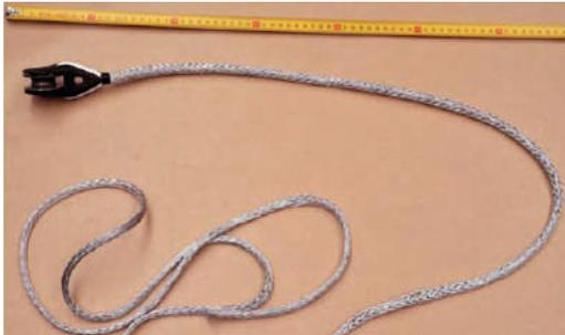
12/ Add lubricant to Dyneema<sup>®</sup> cover which is in contact with the sheave. Apply generously (INO-ROPE grease).
