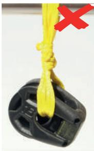
Missing half hitches on lashing (one per extremity instead of 3 per extremity)
